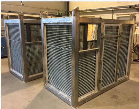
Custom recovery baskets designed for offshore lifting
