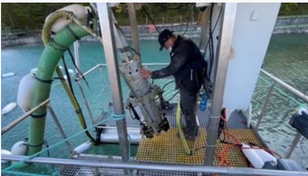
Dredging barge and suction arrangement in operation
