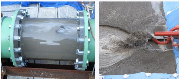
Sediment discharge during testing
