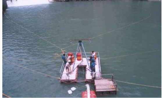
SediCon HydroSuction Dredge operating at Malana reservoir
