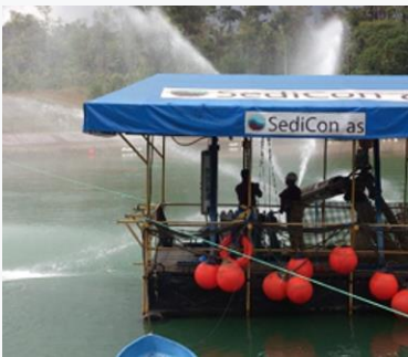
Sediment removal during HydroSuction Dredge operation
