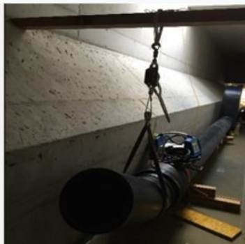
Ø355 SediCon Sluicer installed in the desander
