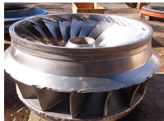
d) Wear of a Francis turbine, Chile
