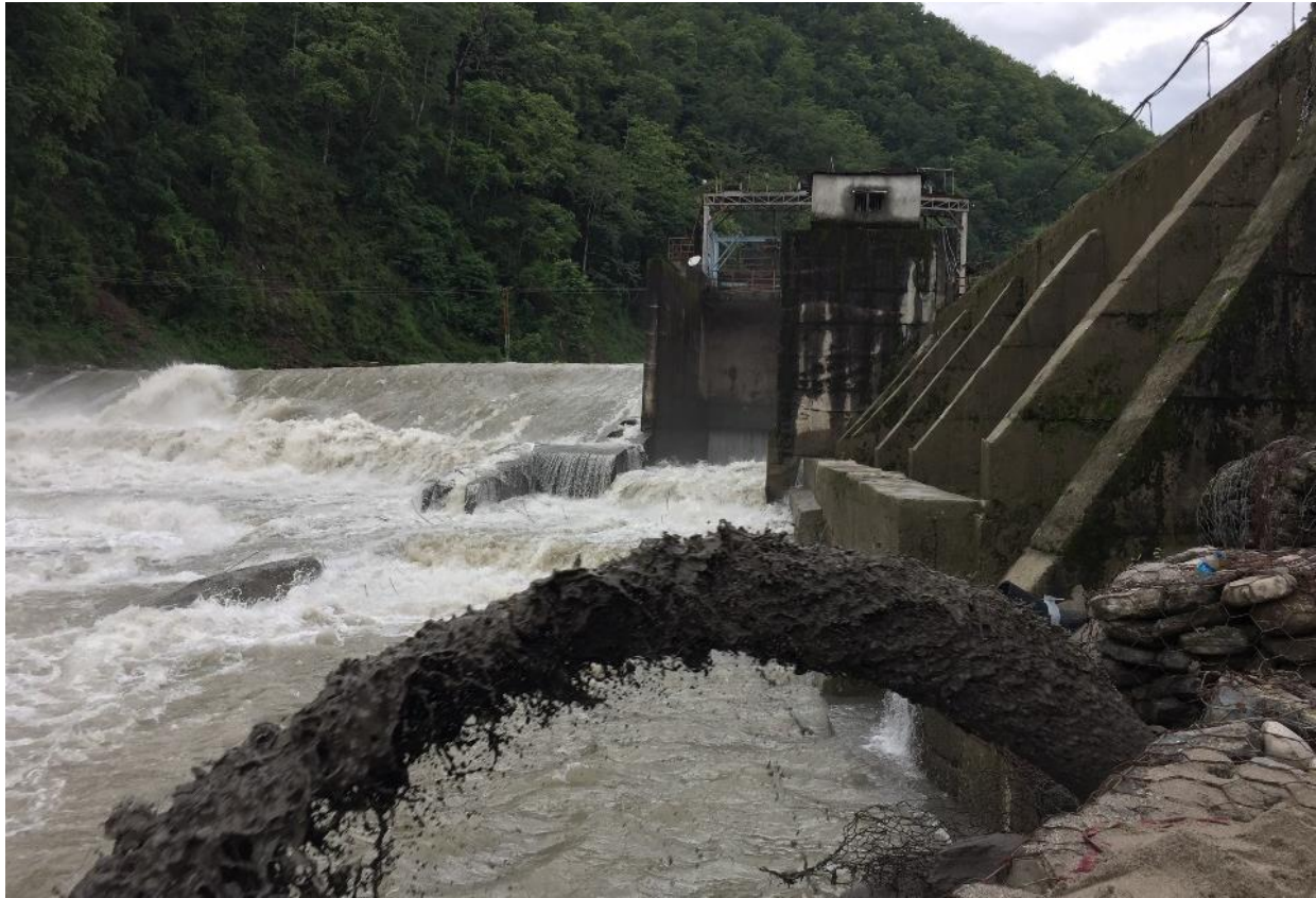
Fig. 6 Discharge from SediCon Sluicer unit 1, 1,480 ton of sand per hour. The discharge of sand equals well above one barrel of sand every second.
